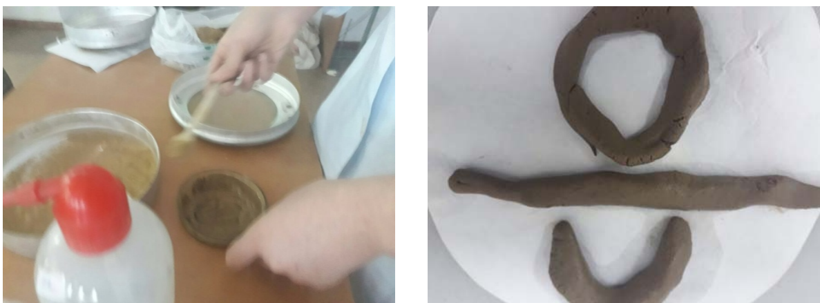
Figure 4 – Soil sample necessary to detect mechanical composition by the wet method
