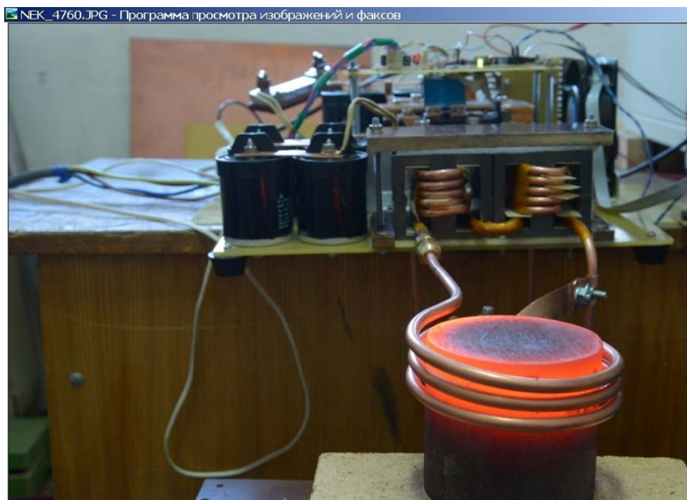
Figure 3 – Process of induction surface heating of metal with a 120 mm diameter at a frequency of 20 kHz
