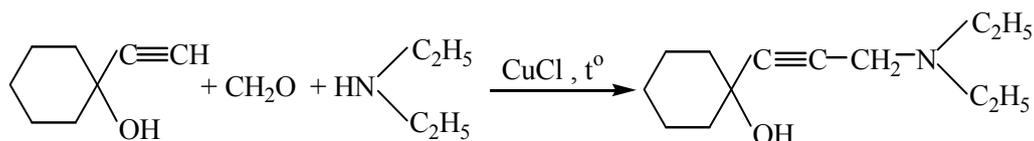
To a three-neck flask with a volume of 1 l, equipped with a mechanical stirrer with an oil shutter, by a reflux condenser and a separating funnel, put 400 ml of dry dioxane, 124 g (1 mol) ethynylcyclohexanol, 9.9 g (0.1 mol) freshly prepared copper monochloride, 30 g of paraform and, stirring, were heated to 70°C.
