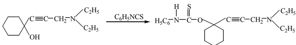
The equimolar amount of the components interacts when heated in the medium of an organic solvent. To do this, in a flask equipped with a reflux condenser were placed 4.18 g (0.02 mol) of acetylene amino alcohol 1-cyclohexyl- (1') -ol-3-diethylamino-propyne-1 and 2.7 g (0.02 mol) of phenyl isothiocyanate in 50 ml of abusolutized benzene, heated at the boiling point of the latter for 5 hours.
